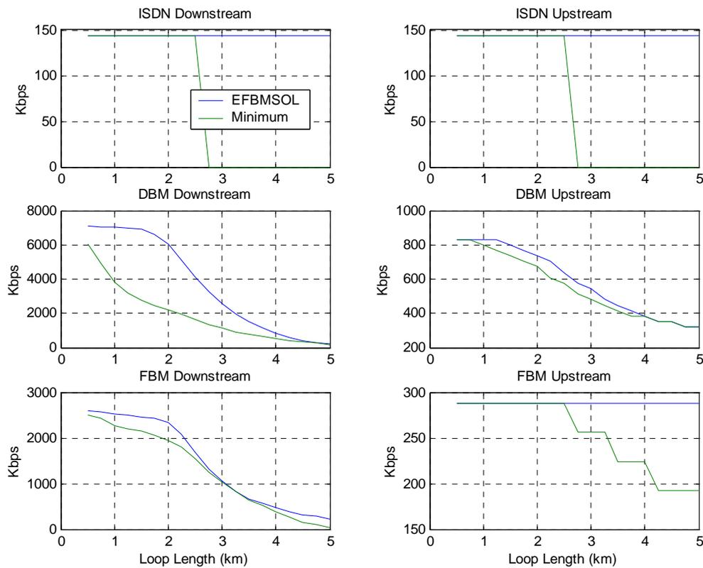
**Figure 5: Spectral Compatibility of Proposed EFBM-sOL**
