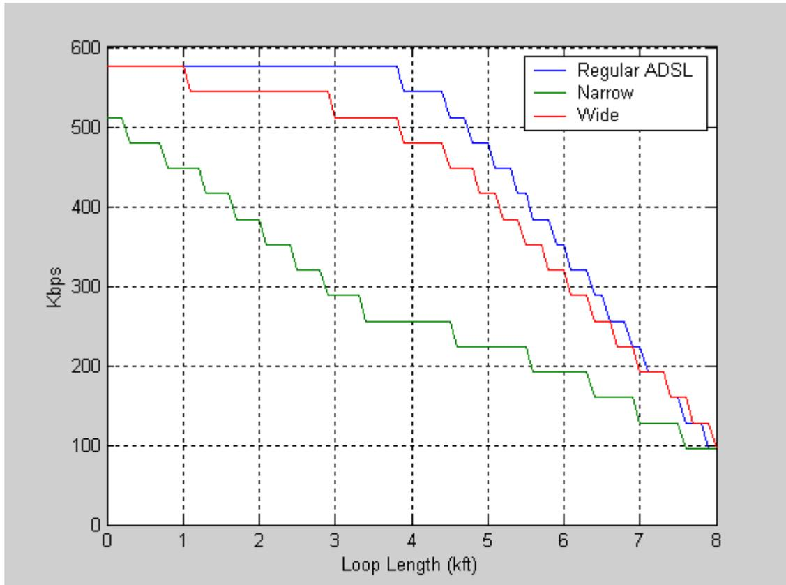
**Figure 4: Upstream Performance of the original FBM-sOL and Annex L Narrow and Wide**
