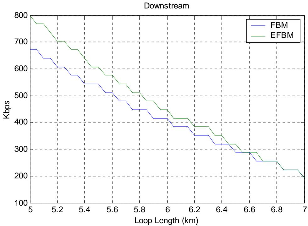
**Figure 3: Downstream Performance of EFBM-sOL and the original FBM-sOL with same quad ISDN crosstalk.**
