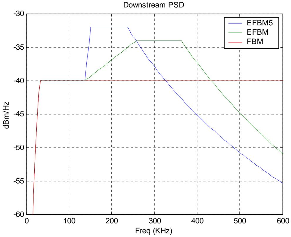
Figure 1: 拡張FBMsOL (EFBMsOL)の下りPSD
