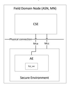
Figure 5.3-1: Secure Environment architecture in a Field Domain Node
