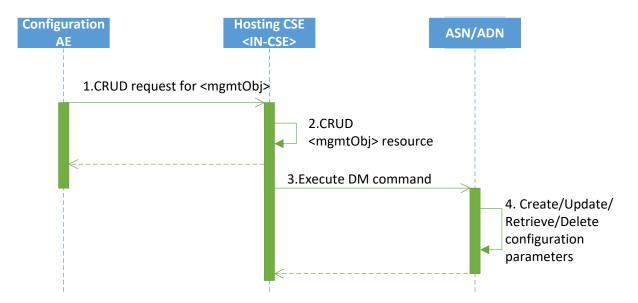
Figure 8.1.3.2-1: Management using Device Management technologies
