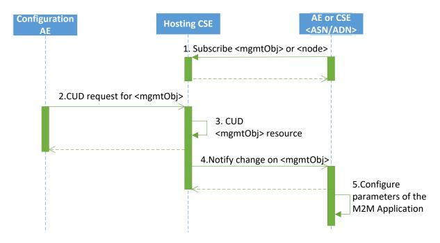
Figure 8.1.3.3-1: Management using the Mcc reference point
