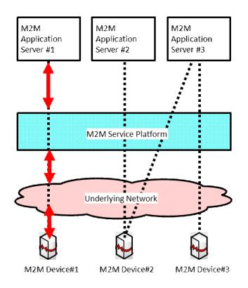
Figure 12.2.9-1 High Level Illustration of Data Traffic Management by Underlying Network Operator
