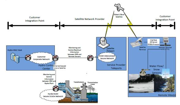
Figure 5.4.9-1 High Level Illustration of Environmental Monitoring for Hydro-Power Generation using Satellite M2M
