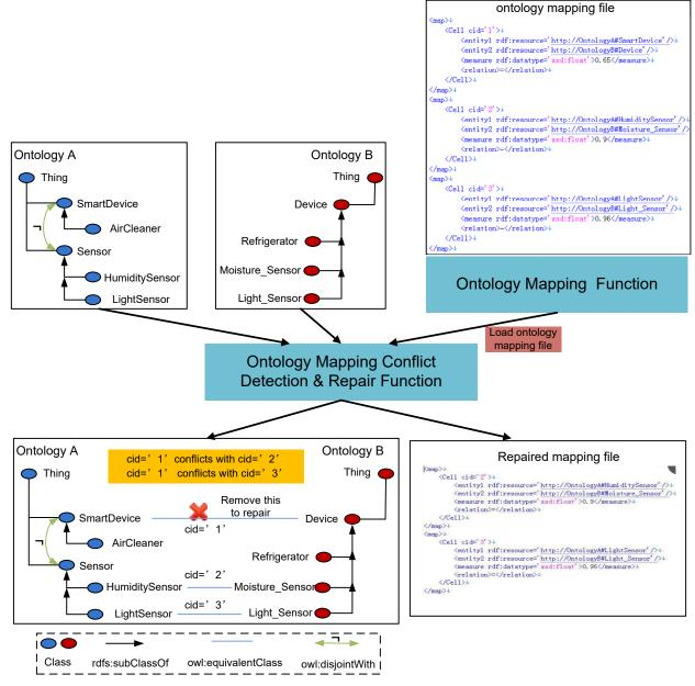
Figure 12.24.9-1 Ontology mapping conflict detection and repair – High-level Illustration
