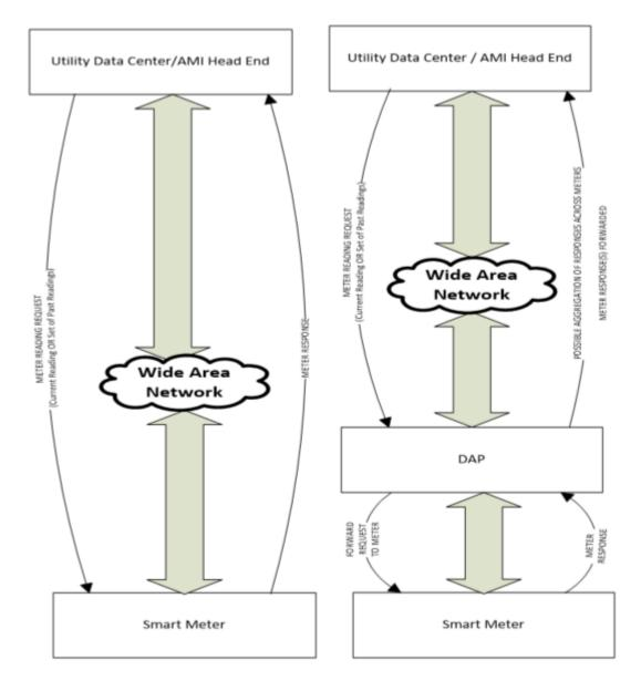
Figure 5.3.6-2 Typical Smart Meter Reading Flows A (on left) and B (on right)
