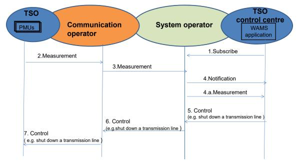
Figure 5.1.6-1 An example flow for the TSO scenario
