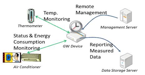
Figure 9.5.9-1 Event triggered Task Execution High Level Illustration
