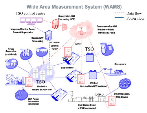
Figure 5.1.9-1 High Level Illustration of Wide Area Measurement System
