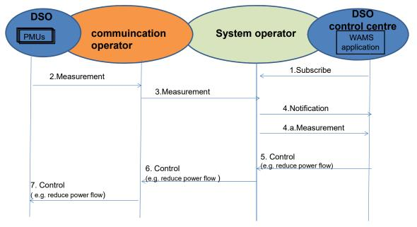
Figure 5.1.6-2 An example flow for DSO scenario
