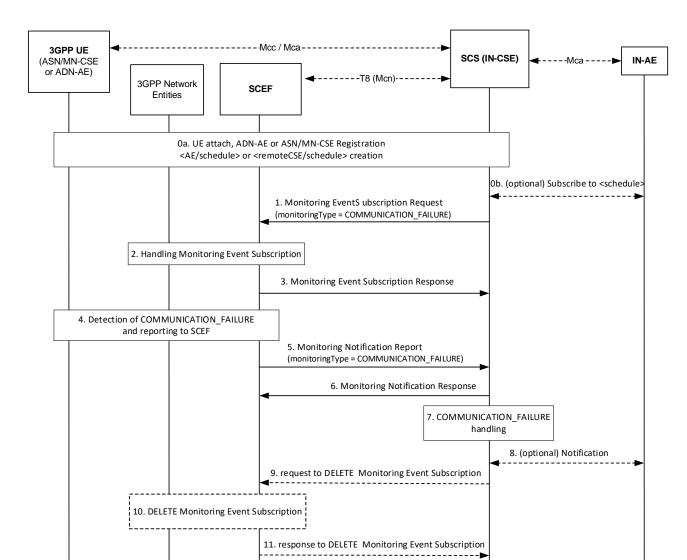
Figure 7.4.3 -1: Communication Failure monitoring
