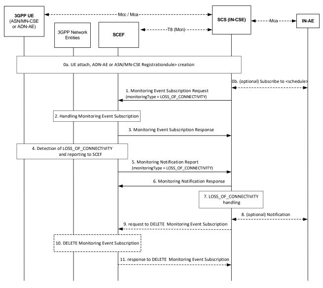
Figure 7.4.4-1: Loss of Connectivity monitoring
