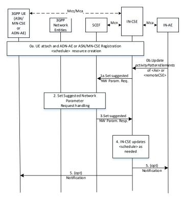
Figure 7.12 -1: Network Parameter Configuration flow
