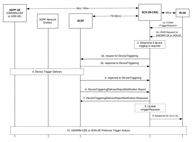
Figure 7.5.1-1: General Procedure for Device Triggering
