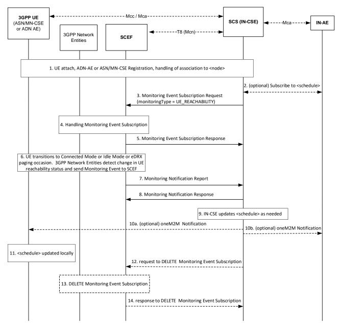
Figure 7.4.1 -1: Procedure for UE Reachability monitoring
