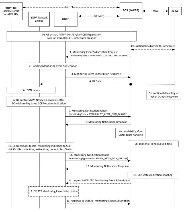
Figure 7.4.2-1: Availability after DDN Failure monitoring
