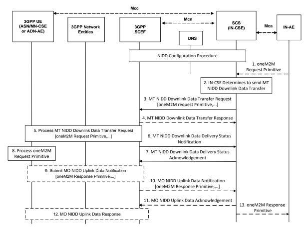
Figure 7.1.1.2-1: SCEF-based Mobile Terminated NIDD
