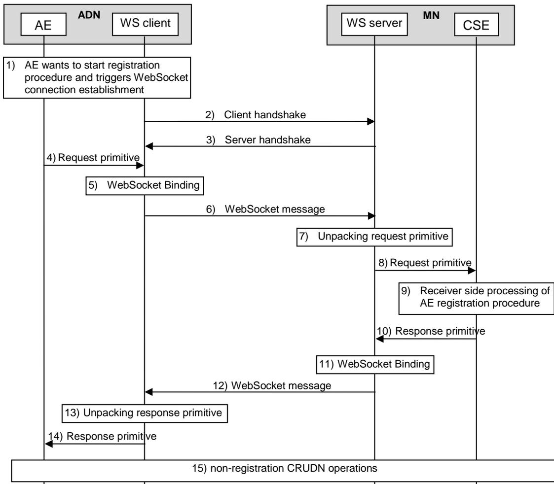
**Figure 5.2-2: Example message flow with WebSocket binding**
