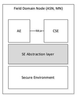
Figure 5.1-1: Secure Environment interworking on Field Domain Node
