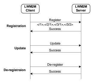
Figure A.5.3.2-1: Example of Registration Procedure
