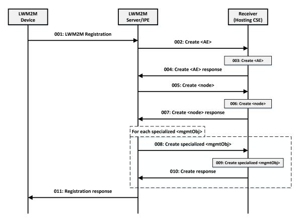
Figure 9.2.2.4-1: End-to-end LWM2M Interworking Procedure
