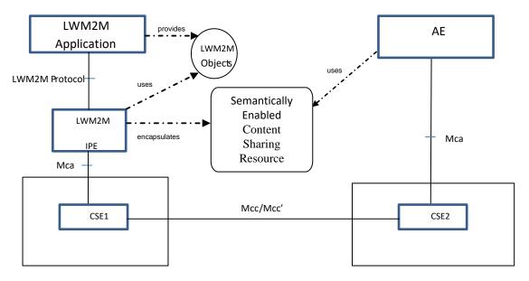
Figure 5.3-2: LWM2M Semantically Enabled Interworking Function
