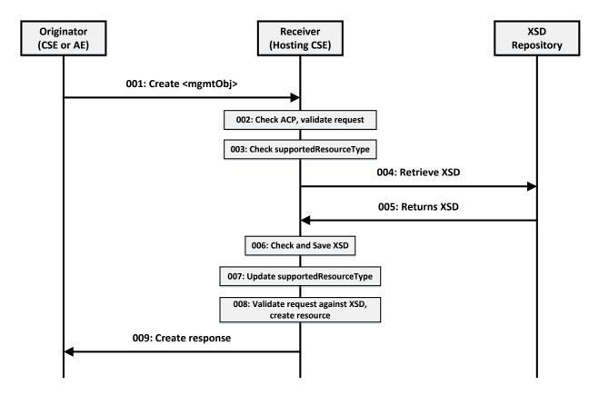
Figure 9.2.2.3-1: Procedure for CSE to Support New Specialized <mgmtObj> Resources
