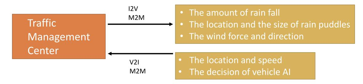
TMC can send location data of the rain puddles etc., but the driver can not use these data for their action. On the other hand, TMC can receive the actual reaction of vehicle by V2I such as the decision parameter of the vehicle at certain rain puddle. However, most of the road authorities are not ready to prepare for constructing data base to assist Automated Vehicles.
