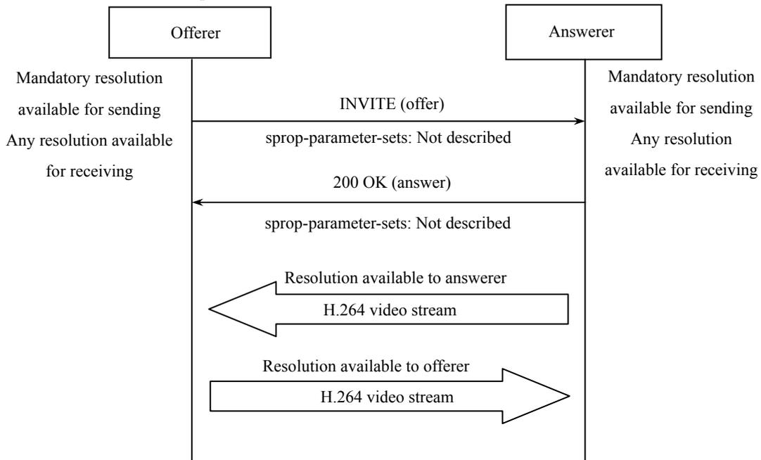
Figure B-6/JJ-40.30: When the offerer and answerer can send video of the mandatory resolution and receive video of any resolution
