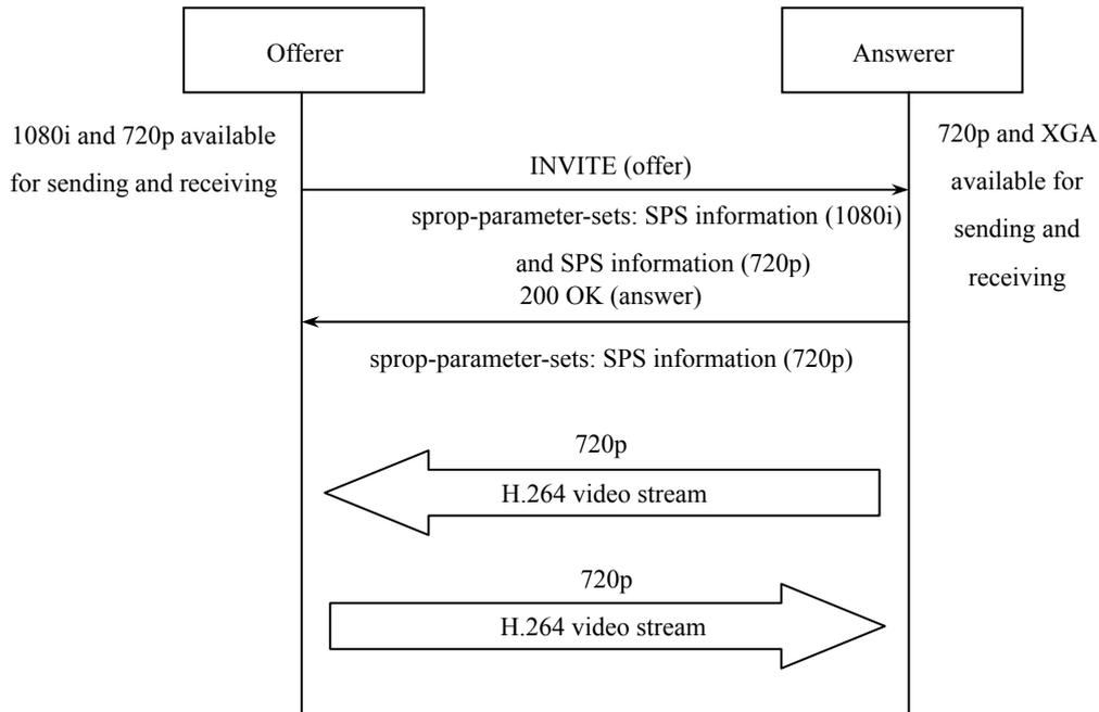
Figure B-3/JJ-40.30: When the offerer and answerer share a resolution available for sending and receiving (example 3)
