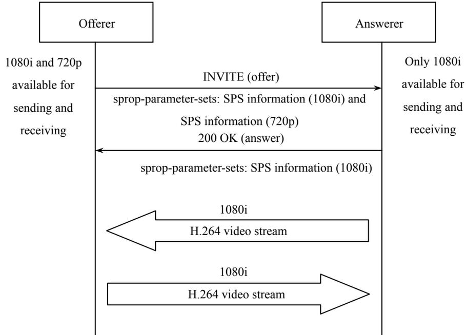
Figure B-2/JJ-40.30: When the offerer and answerer share a resolution available for sending and receiving (example 2)
