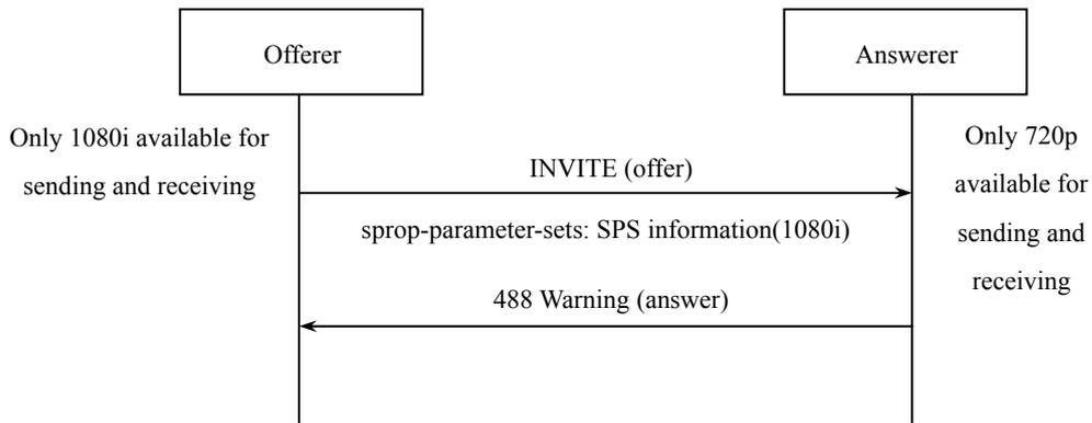
Figure B-7/JJ-40.30: When offerer and answerer do not share any resolution available for sending and receiving
