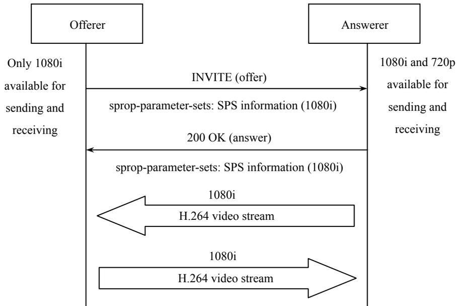
Figure B-1/JJ-40.30: When the offerer and answerer share a resolution available for sending and receiving (example 1)
