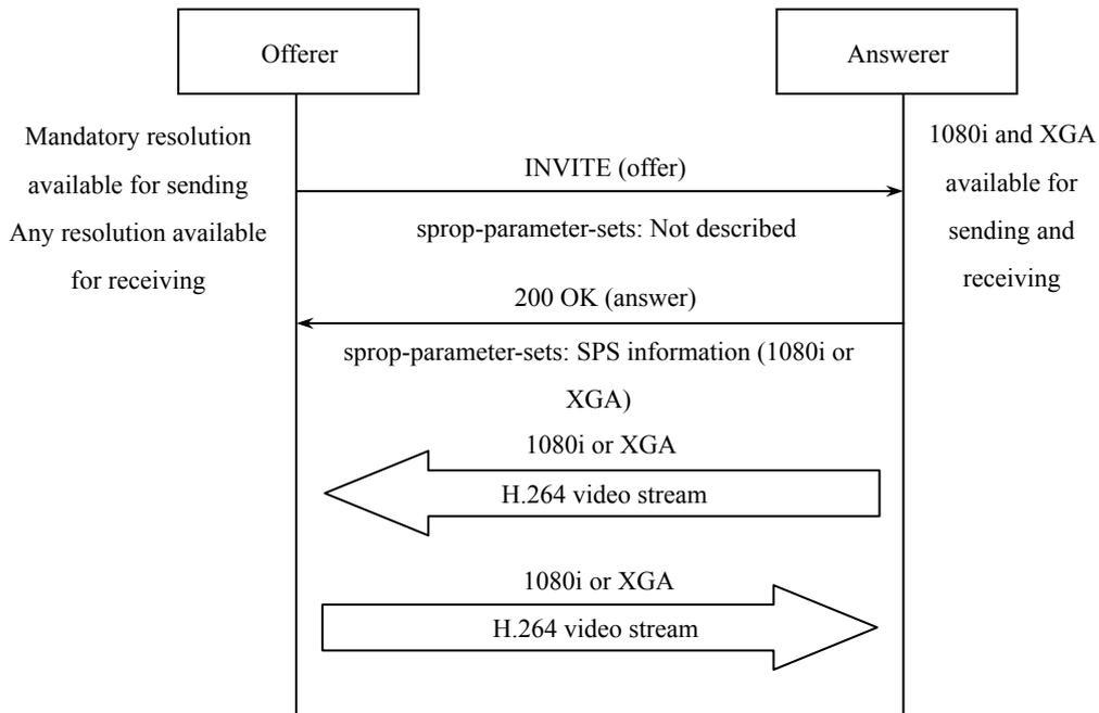
Figure B-4/JJ-40.30: When the offerer can send video of the mandatory resolution and receive video of any resolution (example 1)
