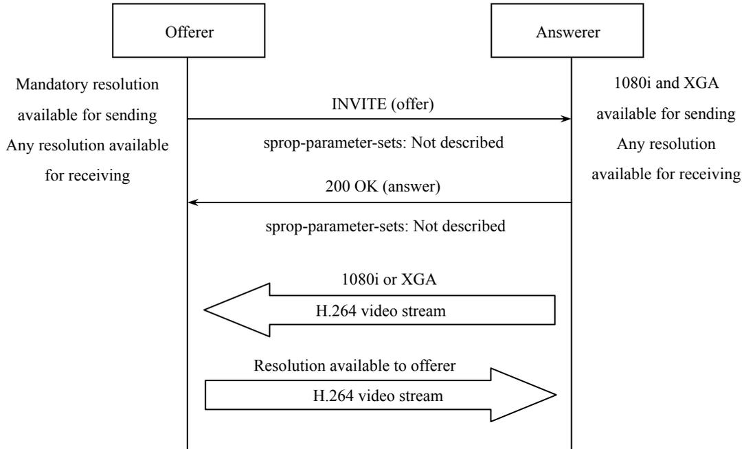
Figure B-5/JJ-40.30: When the offerer can send video of the mandatory resolution and receive video of any resolution (example 2)
