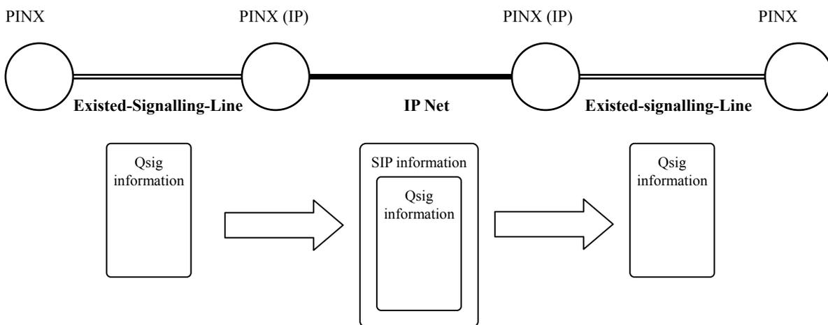
Figure 4-1 Flow of signalling information in ISO/IEC standards
