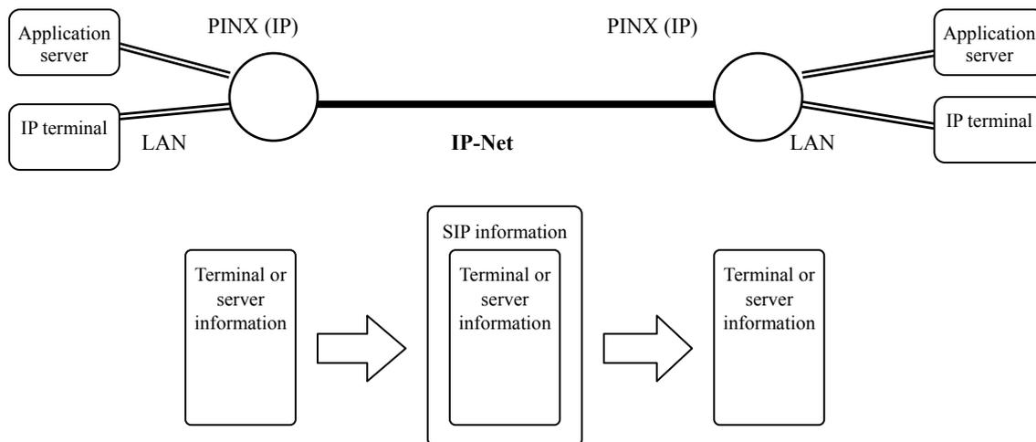
Figure 4-2 Flow of signalling information in the user-specific SIP protocol
