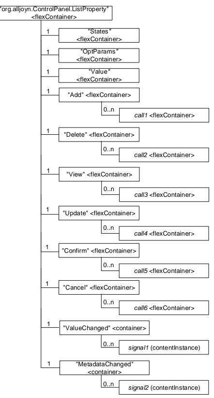
Figure C.2.7-1: Structure of ListProperty interface mapping
