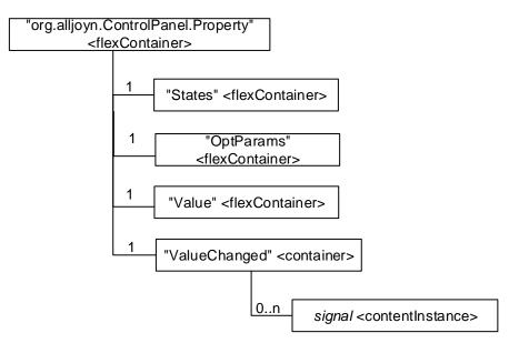
Figure C.2.2-1: Structure of Property interface mapping
