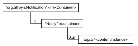
Figure C.1.1-1: Structure of Notification interface mapping
