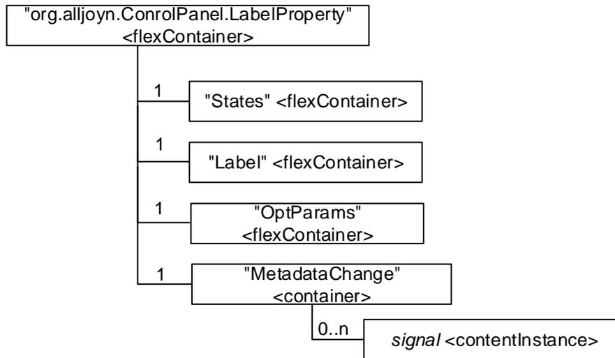
Figure C.2.3-1: Structure of *LabelProperty* interface mapping
