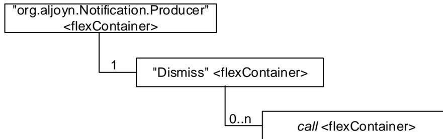
**Figure C.1.2-1: Structure of Notification Producer interface mapping**
