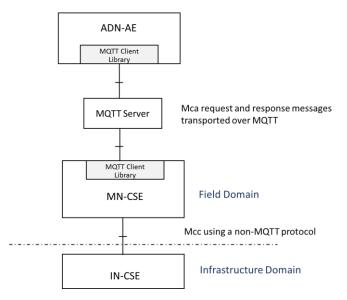
Figure 5.2.3.6-1: Using MQTT between AE and MN-CSE
