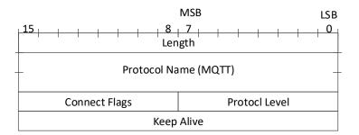
Figure 6.3.1-1: Variable header of MQTT CONNECT Packet
