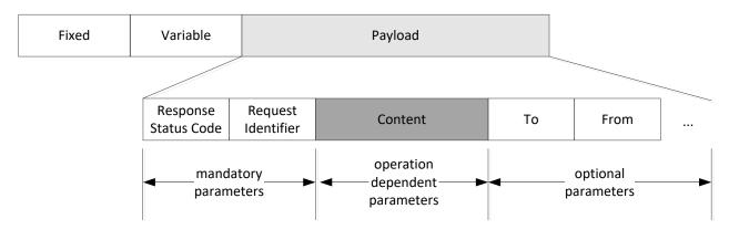
Figure 6.5.2-1: MQTT Response example
