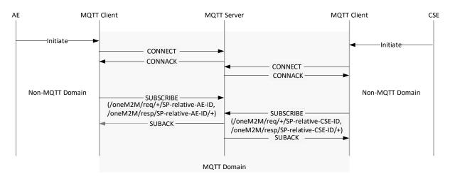
Figure 6.4.5-1: Initiating Process in MQTT binding
