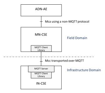
Figure 5.2.3.3-1: Mcc using MQTT between MN and IN
