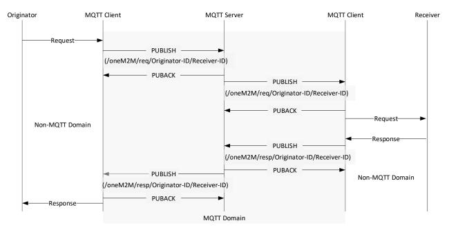
Figure 6.4.5-2: Request/Response message delivery over MQTT
