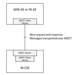
Figure 5.2.3.1-1: Using MQTT between AE and IN-CSE
