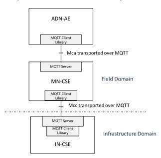
Figure 5.2.3.4-1: Mca and Mcc both using MQTT
