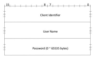
Figure 6.3.2-1: Example of an MQTT CONNECT Packet
