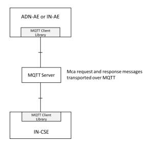
Figure 5.2.3.5-1: Using MQTT between AE and IN-CSE
