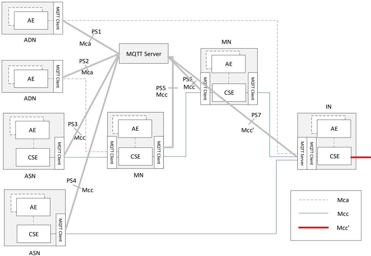
**Figure 5.2.2.2-1: MQTT server independently-located scenario**
