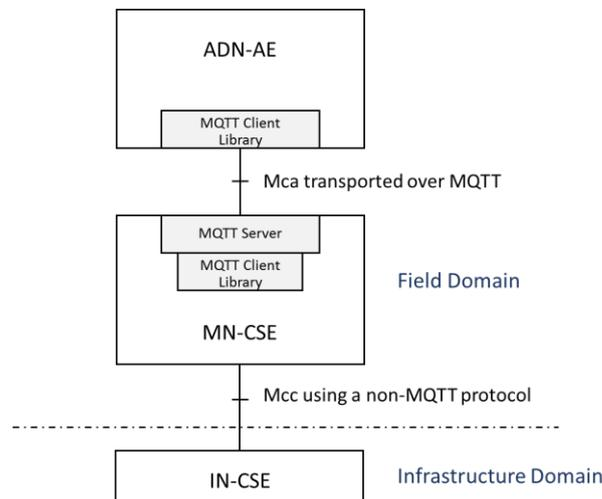
**Figure 5.2.3.2-1: Using MQTT between AE and MN-CSE**
