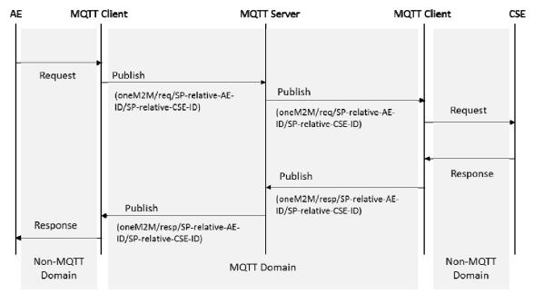
Figure 6.4.5-2: Request/Response message delivery over MQTT
