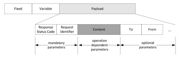
Figure 6.5.2-1: MQTT Response example
