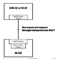
Figure 5.2.3.1-1: Using MQTT between AE and IN-CSE
