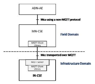
Figure 5.2.3.3-1: Mcc using MQTT between MN and IN
