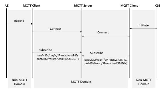
Figure 6.4.5-1: Initiating Process in MQTT binding
