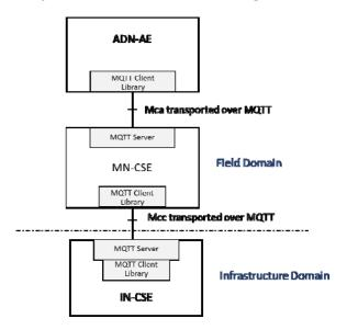
Figure 5.2.3.4-1: Mca and Mcc both using MQTT
