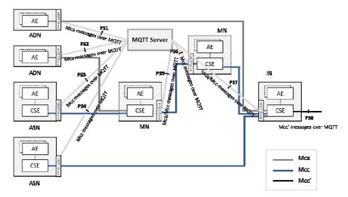
Figure 5.2.2.2-1: MQTT server independently located scenario
