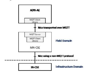
Figure 5.2.3.2-1: Using MQTT between AE and MN-CSE
