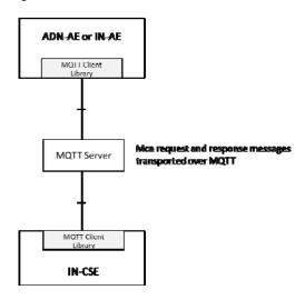
Figure 5.2.3.5-1: Using MQTT between AE and IN-CSE
