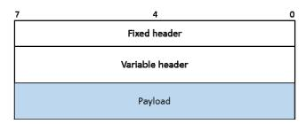
Figure 6.4.1-1: Message format of MQTT Control Packet
