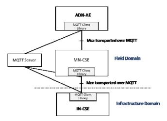
Figure 5.2.3.8-1: Mca and Mcc both using MQTT
