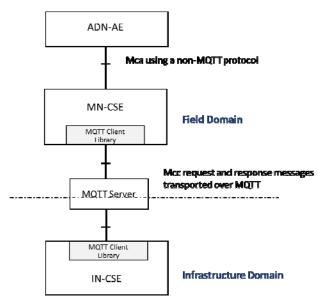
Figure 5.2.3.7-1: Mcc using MQTT between MN and IN
