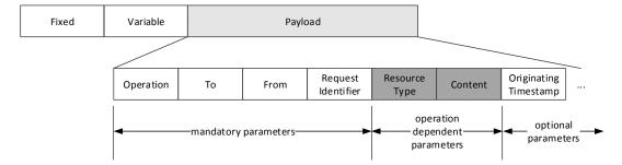
Figure 6.5.1-1: MQTT Request example
