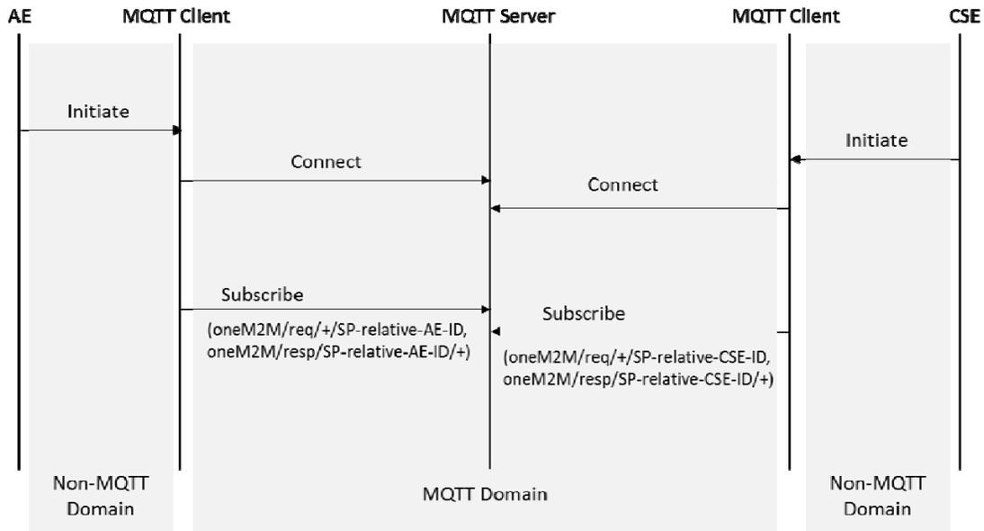
**Figure 6.4.5-1: Initiating Process in MQTT binding**
