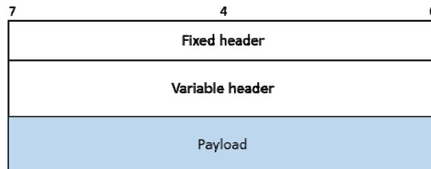
Figure 6.4.1-1: Message format of MQTT Control Packet
