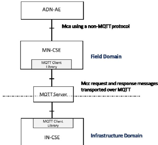
**Figure 5.2.3.7-1: Mcc using MQTT between MN and IN**
