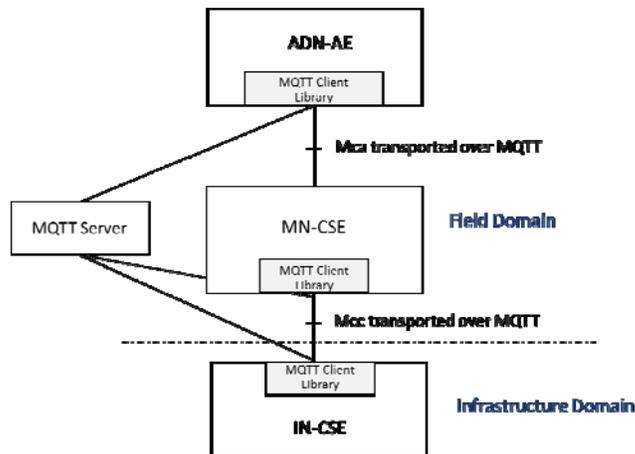
**Figure 5.2.3.8-1: Mca and Mcc both using MQTT**
