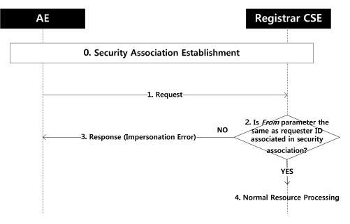
Figure 7.2-1: AE impersonation checking procedure
