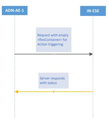
Figure 8.3.3.4-1: Action triggering procedure
