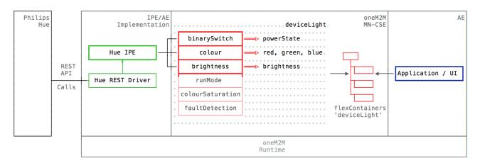
Figure 9.1-1: Implementation of TS-0023 [i.2] Module Classes for the Hue bulb use case
