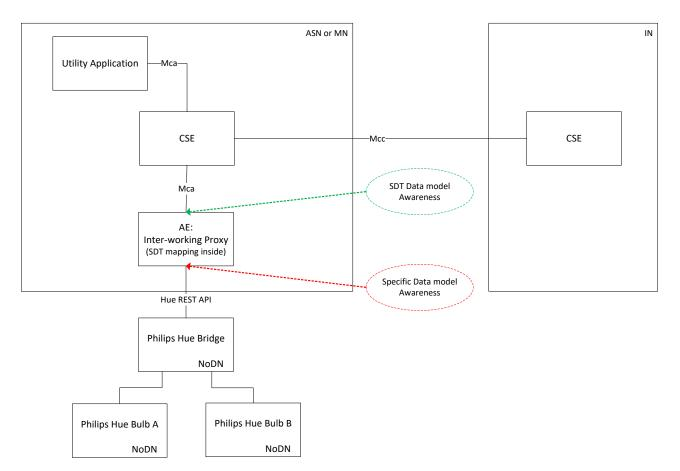
Figure 6.3-1: Translation of non-oneM2M Data Model to SDT Data Model via the IPE
