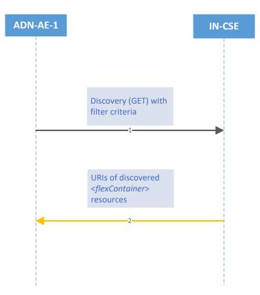
Figure 8.3.2-1: Discovery of SDT Device with filter criteria
