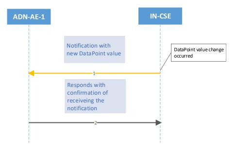
Figure 8.3.3.5-3: Notification mechanism procedure
