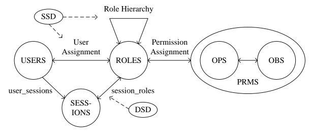
Figure 3: Role based access control model
