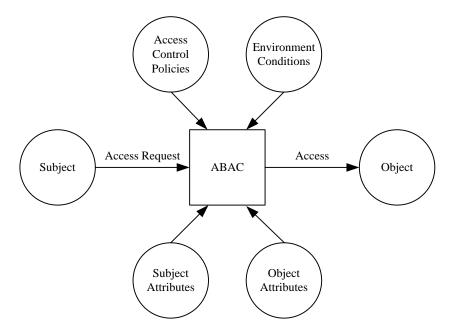
Figure 4: Attribute based access control model
