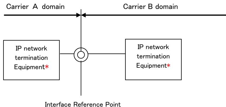
\* The equipments enable transmission and termination using Layer 1 and Layer 2 functions.
