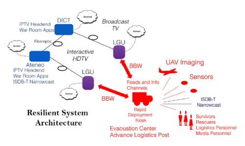
Figure 2-5-1: Future Wireless System for Pre-Disaster Preparation and Post Disaster Rescue and Recovery
