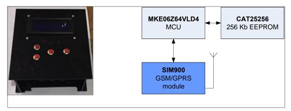
Figure 2-6-3: Block diagram of the processing components inside a MMC device
