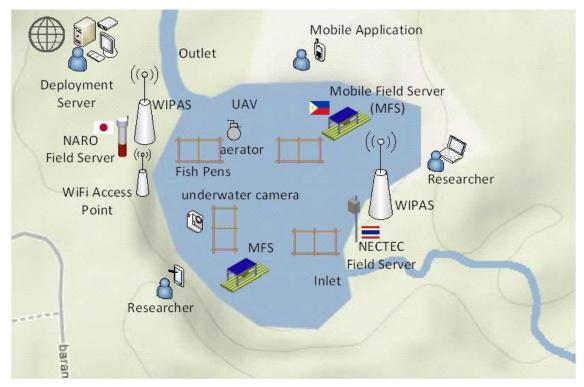
Figure 2-1-4: System configuration in Palakpakin lake
