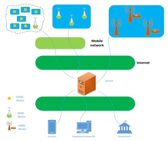
Figure 2-6-1: Overall architecture of proposed system
