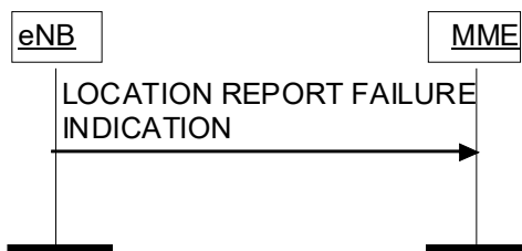
Figure 8.11.2.2-1: Location Report Failure Indication procedure.
