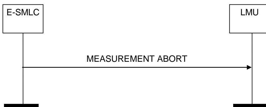
Figure 8.2.3.2.1: Measurement Abort Procedure: Successful Operation.
