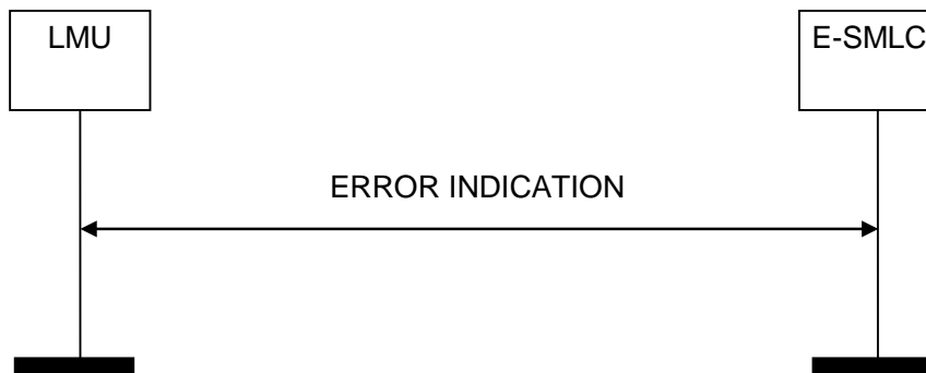
Figure 8.3.3.2.1: Error Indication procedure
