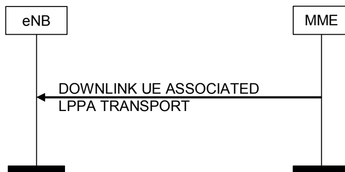
Figure 8.17.2.1-1: DOWNLINK UE ASSOCIATED LPPA Transport Procedure
