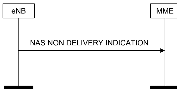
Figure 8.6.2.4-1: NAS NON DELIVERY INDICATION Procedure
