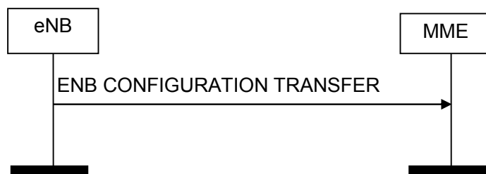
Figure 8.15.2.1-1: eNB Configuration Transfer procedure. Successful operation.
