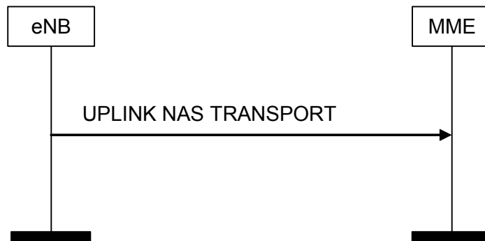
Figure 8.6.2.3-1: UPLINK NAS TRANSPORT Procedure
