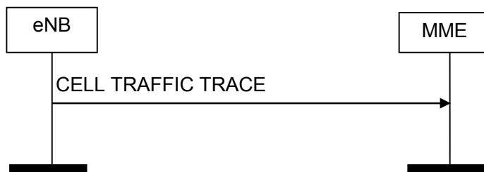
Figure 8.10.4.2-1: Cell Traffic Trace procedure. Successful operation.
