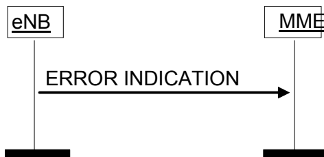
Figure 8.7.2.2-2: Error Indication procedure, eNB originated. Successful operation.
