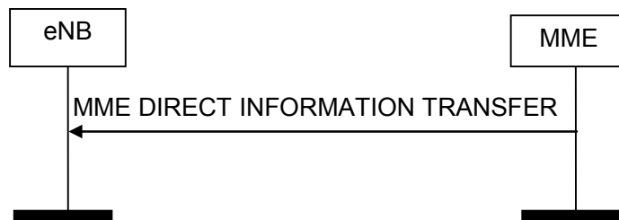
Figure 8.14.1.2-1: MME Direct Information Transfer procedure. Successful operation.
