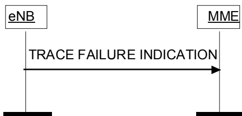
Figure 8.10.2.2-1: Trace Failure Indication procedure.
