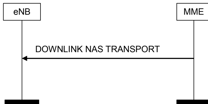
Figure 8.6.2.2-1: DOWNLINK NAS Transport Procedure
