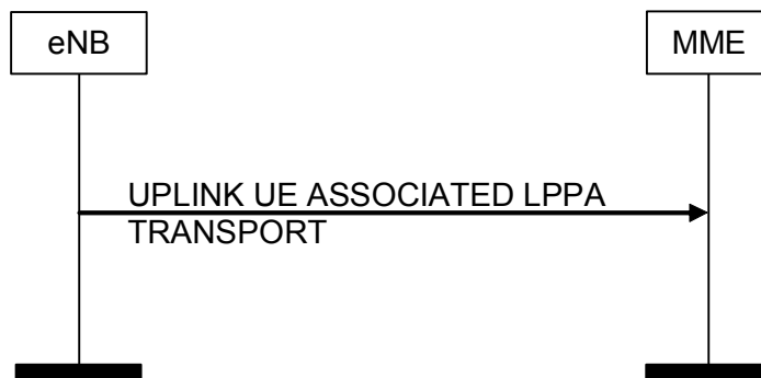
Figure 8.17.2.2-1: UPLINK UE ASSOCIATED LPPA TRANSPORT Procedure
