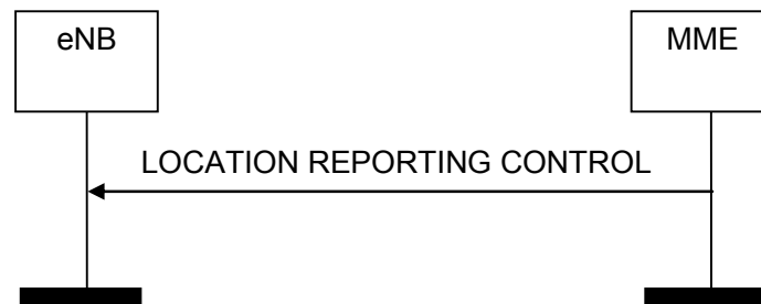
Figure 8.11.1.2-1: Location Reporting Control procedure. Successful operation.
