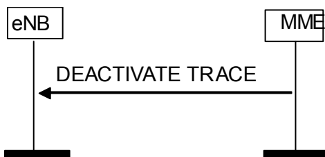
Figure 8.10.3.2-1: Deactivate Trace procedure. Successful operation.
