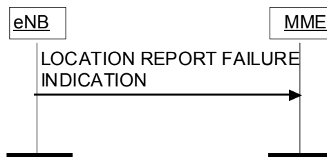
Figure 8.11.2.2-1: Location Report Failure Indication procedure.
