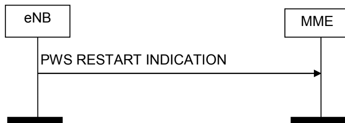
Figure 8.12.3.2-1: PWS Restart Indication procedure. Successful operation.
