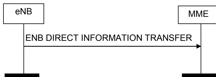
Figure 8.13.1.2-1: ENB Direct Information Transfer procedure. Successful operation.
