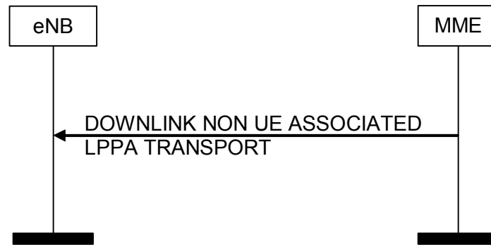
Figure 8.17.2.3-1: DOWNLINK NON UE ASSOCIATED LPPA Transport Procedure
