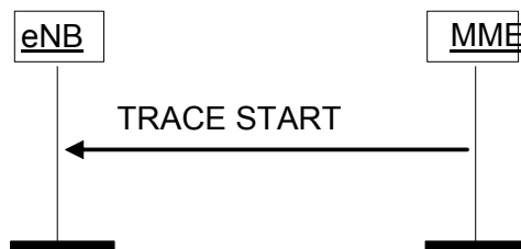
Figure 8.10.1.2-1: Trace Start procedure.
