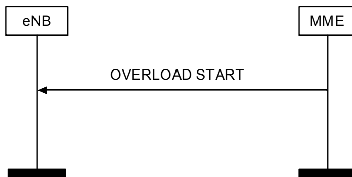
Figure 8.7.6.2-1: Overload Start procedure
