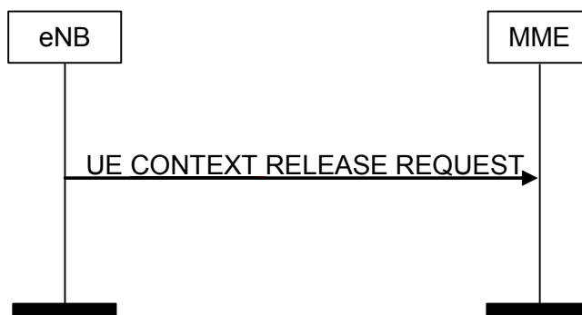
Figure 8.3.2.2-1: UE Context Release Request procedure. Successful operation.
