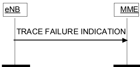
Figure 8.10.2.2-1: Trace Failure Indication procedure.
