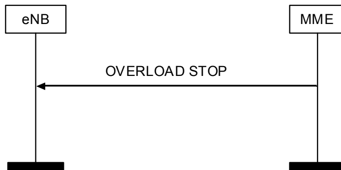
Figure 8.7.7.2.-1: Overload Stop procedure
