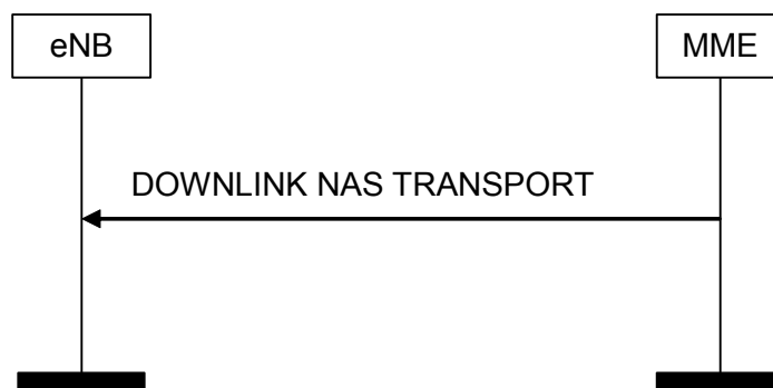
Figure 8.6.2.2-1: DOWNLINK NAS Transport Procedure
