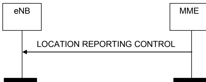
Figure 8.11.1.2-1: Location Reporting Control procedure. Successful operation.
