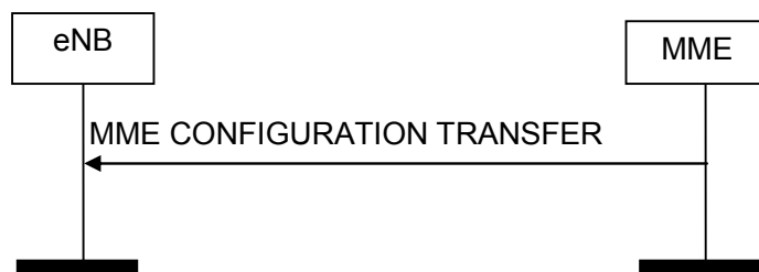
Figure 8.16.2.1-1: MME Configuration Transfer procedure. Successful operation.
