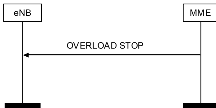
Figure 8.7.7.2.-1: Overload Stop procedure
