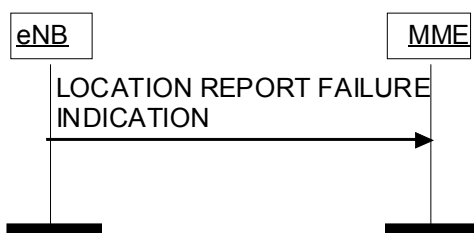
Figure 8.11.2.2-1: Location Report Failure Indication procedure.
