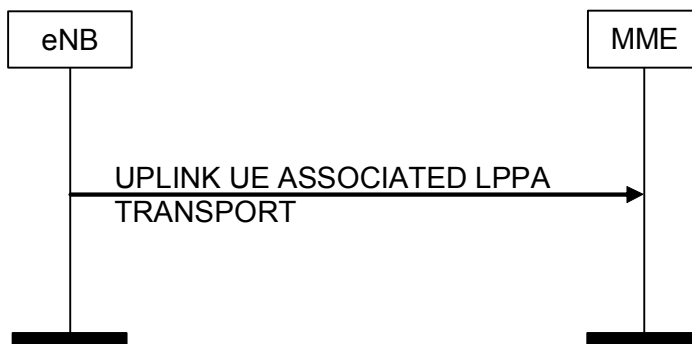
Figure 8.17.2.2-1: UPLINK UE ASSOCIATED LPPA TRANSPORT Procedure
