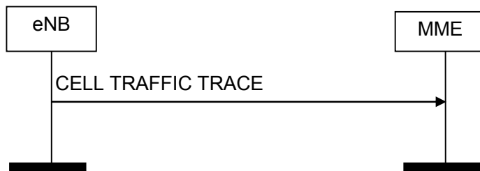
Figure 8.10.4.2-1: Cell Traffic Trace procedure. Successful operation.
