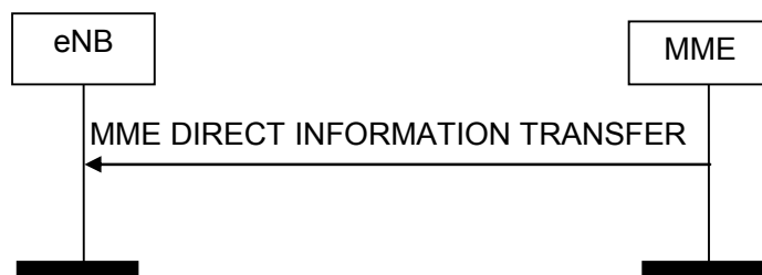
Figure 8.14.1.2-1: MME Direct Information Transfer procedure. Successful operation.
