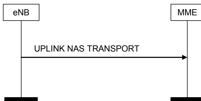
Figure 8.6.2.3-1: UPLINK NAS TRANSPORT Procedure
