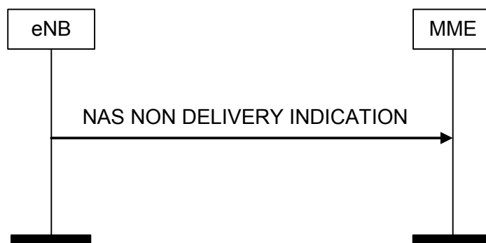
Figure 8.6.2.4-1: NAS NON DELIVERY INDICATION Procedure
