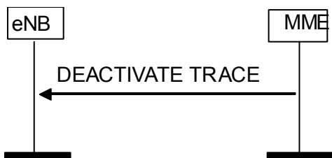
Figure 8.10.3.2-1: Deactivate Trace procedure. Successful operation.
