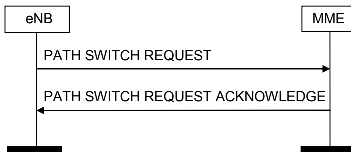
Figure 8.4.4.2-1: Path switch request: successful operation
