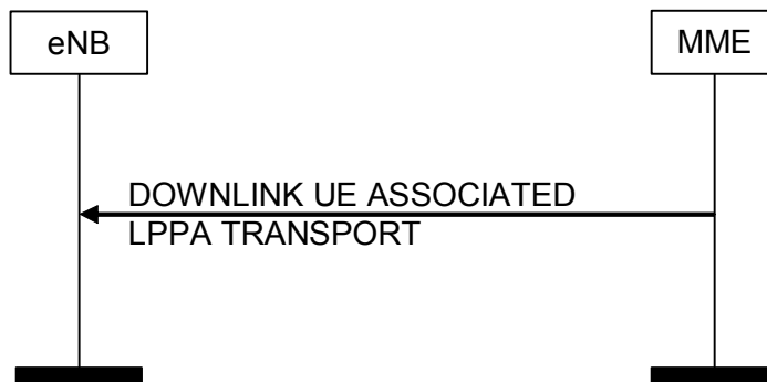
Figure 8.17.2.1-1: DOWNLINK UE ASSOCIATED LPPA Transport Procedure
