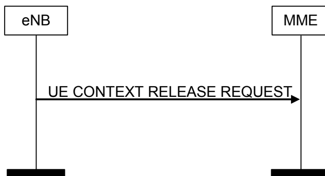
Figure 8.3.2.2-1: UE Context Release Request procedure. Successful operation.
