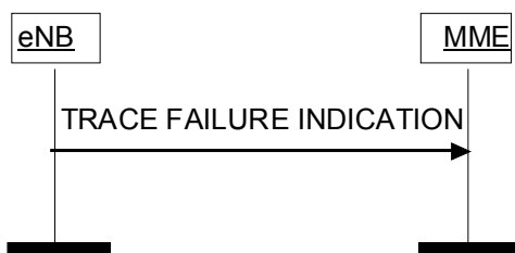
Figure 8.10.2.2-1: Trace Failure Indication procedure.
