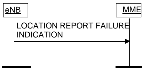
Figure 8.11.2.2-1: Location Report Failure Indication procedure.
