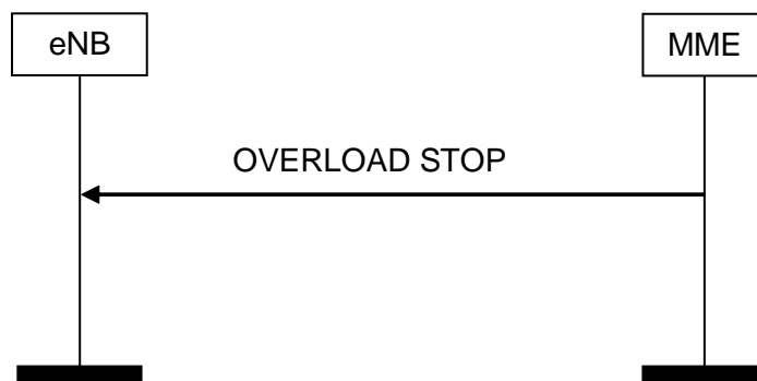
Figure 8.7.7.2.-1: Overload Stop procedure
