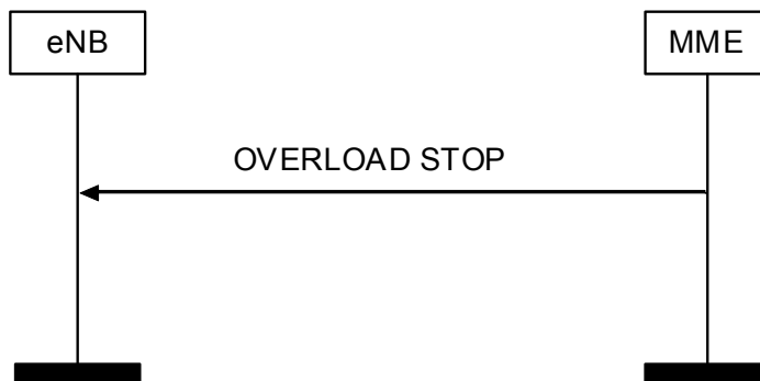
Figure 8.7.7.2.-1: Overload Stop procedure
