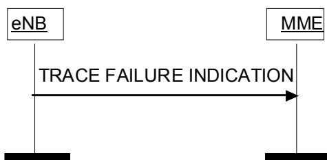
Figure 8.10.2.2-1: Trace Failure Indication procedure.
