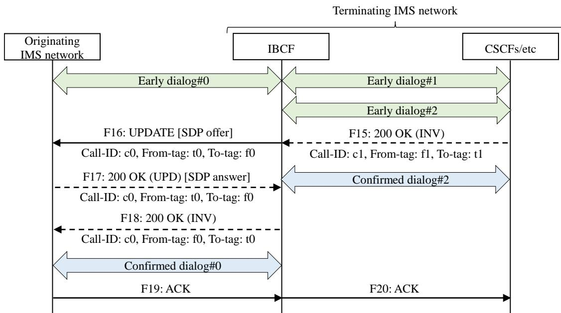
**Appendix Figure vi.2.3-4 / JJ-90.30: Procedure when an IBCF receives a 200 (OK) response to the initial INVITE request not containing SDP**
