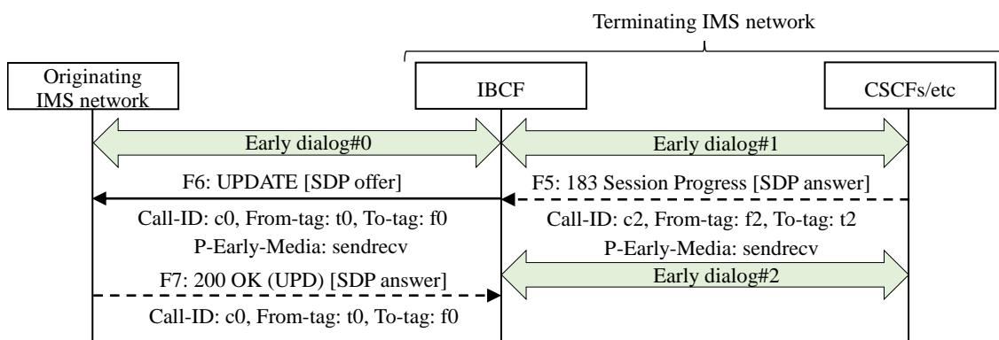
**Appendix Figure vi.2.2.1-2 / JJ-90.30: Procedure when an IBCF receives a subsequent 18x response (IBCF receives an SDP answer and a P-Early-Media header field when the IBCF has sent an SDP answer to the originating IMS network)**
