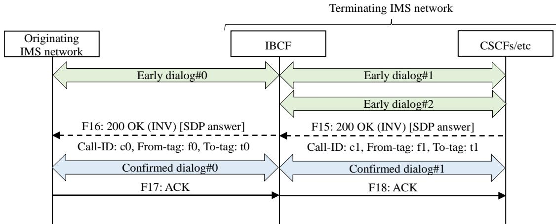
**Appendix Figure vi.2.3-1 / JJ-90.30: Procedure when an IBCF receives a 200 (OK) response containing an SDP answer to the initial INVITE request (the IBCF has not sent the first SDP answer to the originating IMS network)**
