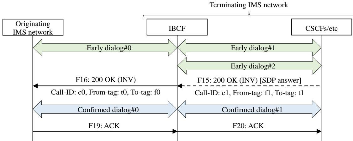
**Appendix Figure vi.2.3-3 / JJ-90.30: Procedure when an IBCF receives a 200 (OK) response containing an SDP to the initial INVITE request**
