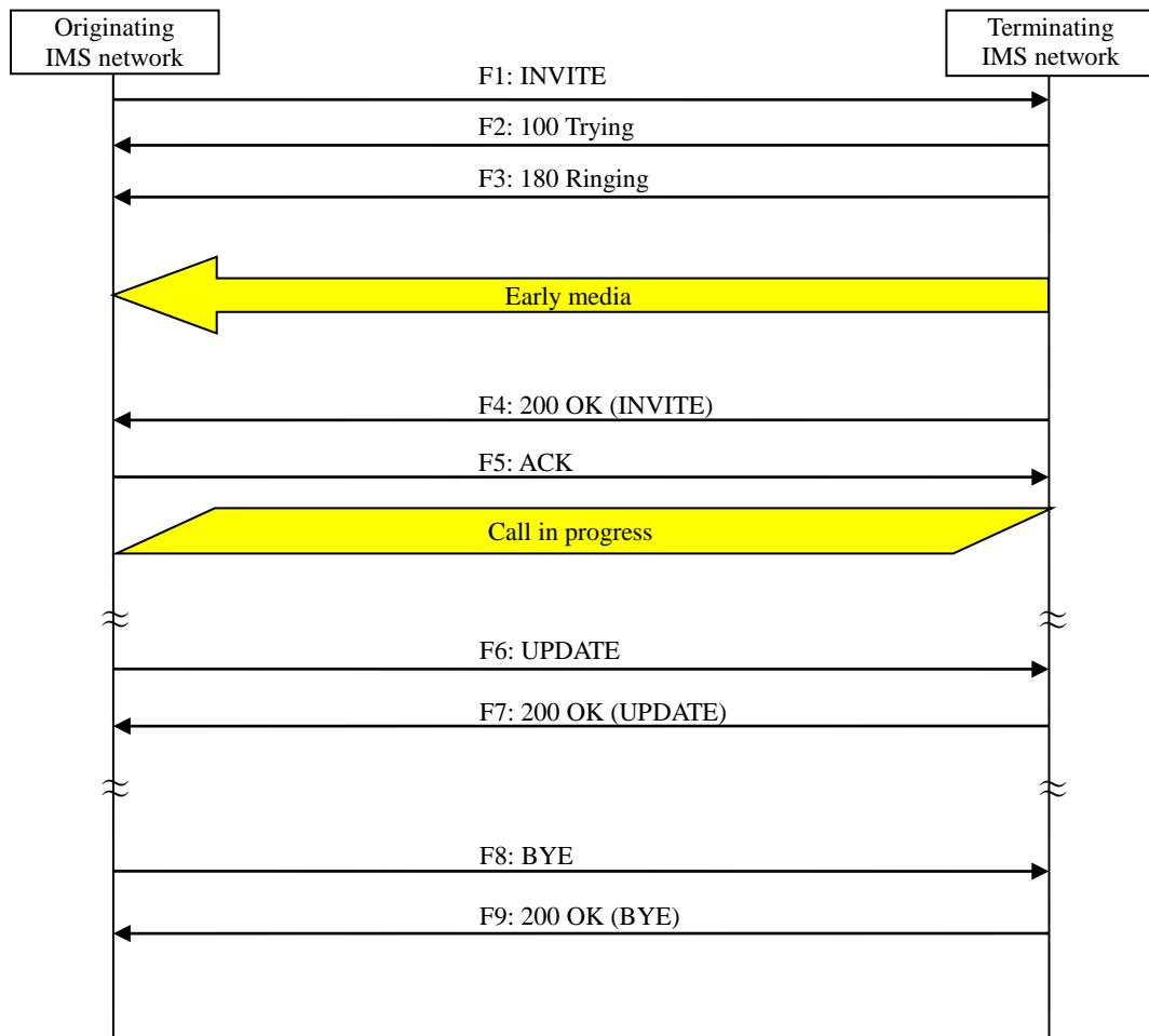
**Appendix Figure vii.2.1.1.2-1 / JJ-90.30: Basic call (Call is released by originating side)(early media) <Originating from fixed IMS network and terminating in fixed IMS network (early media not using "100rel")>**
