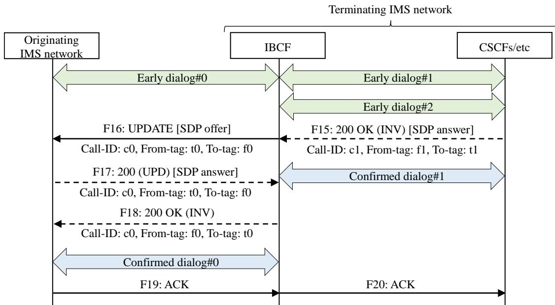
**Appendix Figure vi.2.3-2 / JJ-90.30: Procedure when an IBCF receives a 200 (OK) response containing an SDP to the initial INVITE request**
