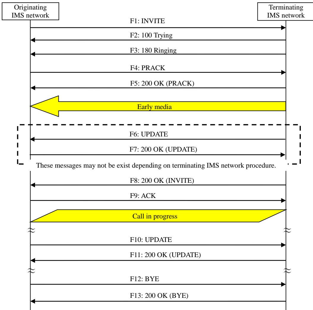
**Appendix Figure 2.1.1.3-1 / JJ-90.30: Basic call (Call is released by originating side)(early media) <Originating from fixed IMS network and terminating in fixed IMS network (early media using gateway model)>**
