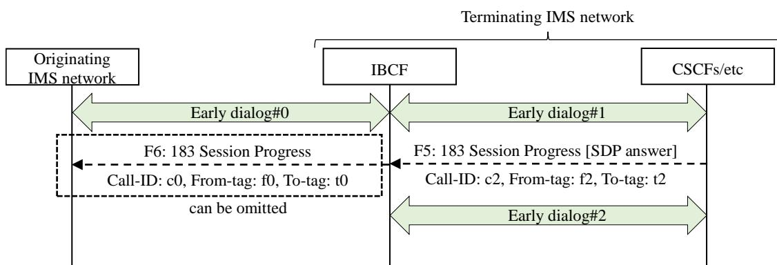
**Appendix Figure vi.2.2.1-3 / JJ-90.30: Procedure when an IBCF receives a subsequent 18x response (IBCF receives an SDP answer and no P-Early-Media header field when the IBCF has sent an SDP answer to the originating IMS network)**
