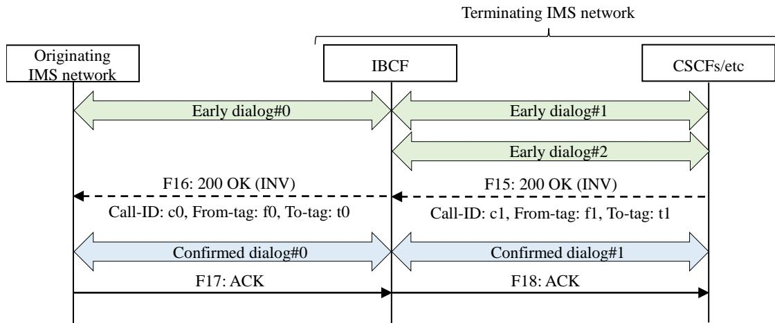
**Appendix Figure vi.2.3-5 / JJ-90.30: Procedure when an IBCF receives a 200 (OK) response to the initial INVITE request not containing SDP**
